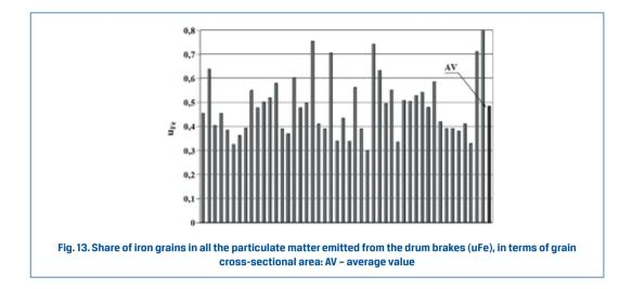
According to the graphs above, the average share of iron grains in all the particulate matter emitted from the brake mechanisms, in terms of grain cross-sectional area, was about 50%.
