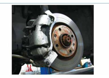
Fig. 3. Disc brake of the Citroen Berlingo vehicle provided with the dust emission reduction system
