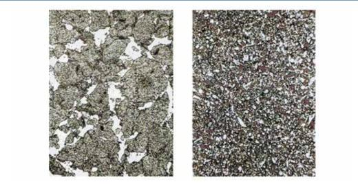
Fig. 9. Dust of the sample taken from the disc brakes; magnitude ×76 (right) and ×910 (left)
