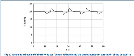
reduce particulate matter emission from passenger car brake mechanisms: v – vehicle speed
