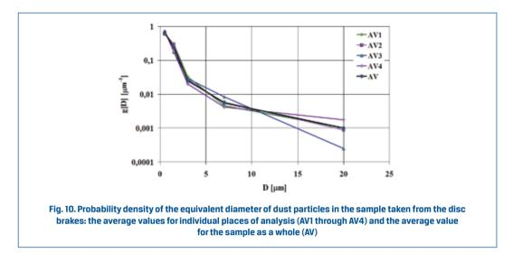
Interestingly, only a small unrepeatability can be observed in the curves determined to represent the probability density of the equivalent dust particle diameter, both for individual analysed places in each of the samples and for the average values for the whole sample. This provides grounds for a statement that the results obtained may be considered reliable and honestly describing the observed properties of the dust samples under examination.
